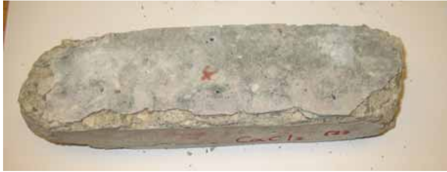
Fig. 9 Specimen subjected to 10 weeks of exposure to a 6.04 molal ion concentration solution of \text{CaCl}_2
