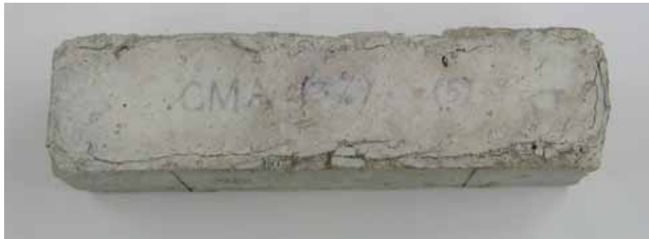
Fig. 7 Specimen subjected to 95 weeks of exposure to a 1.06 molal ion concentration solution of CMA
