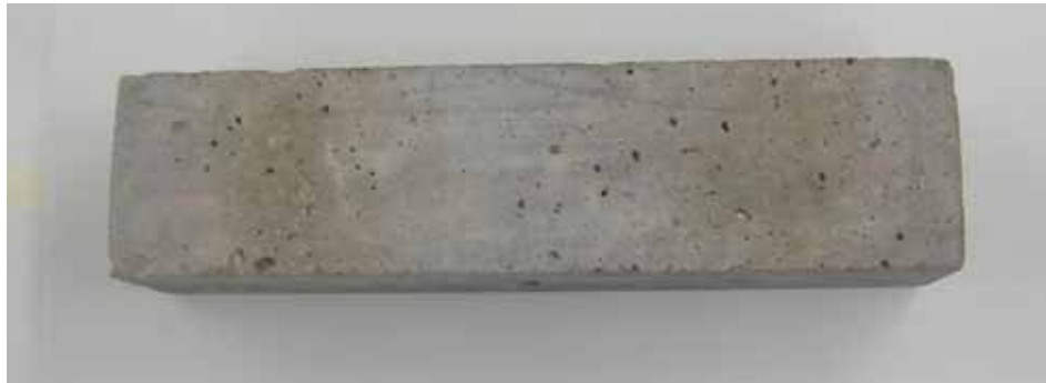
Fig. 5 Specimen subjected to 95 weeks of exposure to a 1.06 molal ion concentration solution of CaCl 2
