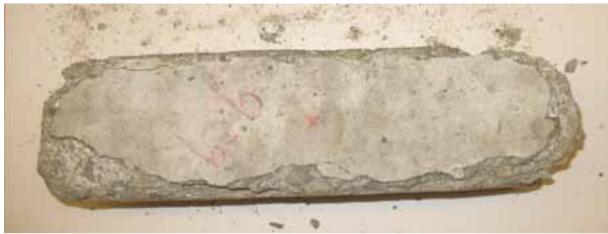
Fig. 10 Specimen subjected to 10 weeks of exposure to a 6.04 molal ion concentration solution of \text{MgCl}_2
