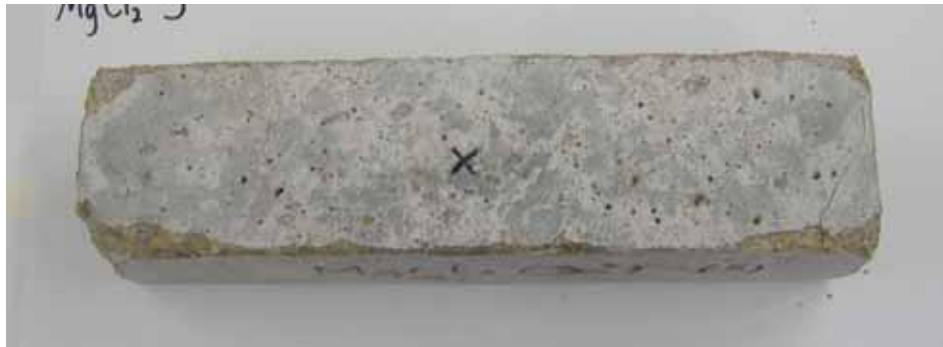
Fig. 6 Specimen subjected to 80 weeks of exposure to a 1.06 molal ion concentration solution of \text{MgCl}_2
