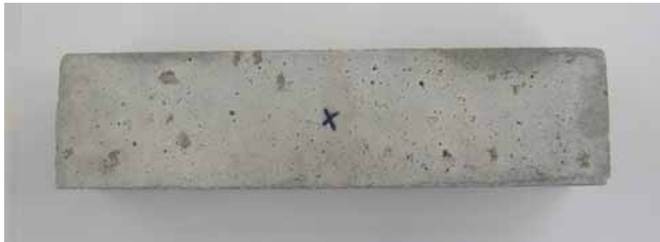
Fig. 4 Specimen subjected to 95 weeks of exposure to a 1.06 molal ion concentration solution of NaCl
