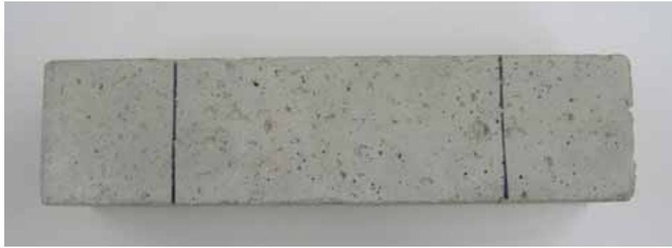
Fig. 3 Specimen subjected to 95 weeks of exposure to distilled water
