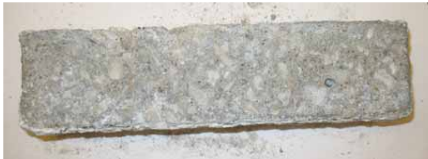
Fig. 11 Specimen subjected to 60 weeks of exposure to a 6.04 molal ion concentration solution of CMA
