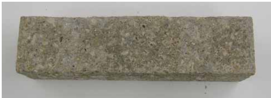
Fig. 8 Specimen subjected to 95 weeks of exposure to a 6.04 molal ion concentration solution of \text{NaCl}
