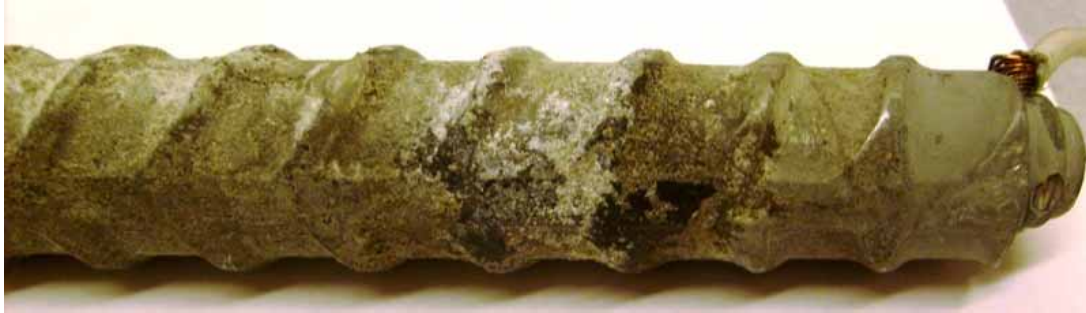
Figure 10 – Specimen B-Zn-45N-4 showing corrosion on the bottom bar
