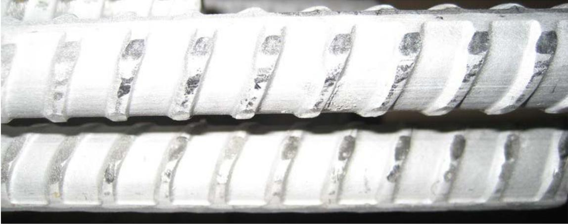
**Figure 1a:** Damage to deformations on straightened XM-28 bars from the straightening process.
