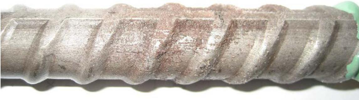
**Figure 20b:** 2205 stainless steel from producer B showing closeup of corrosion products after testing; specimen 2205-3.
