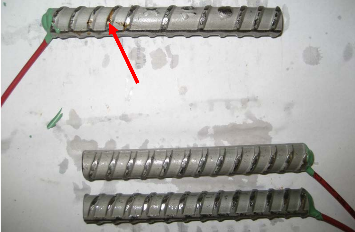
Figure 10a: Straightened XM-28 stainless steel after testing. Anode (top bar) and cathode (bottom bars). Corrosion products indicated with arrow.
