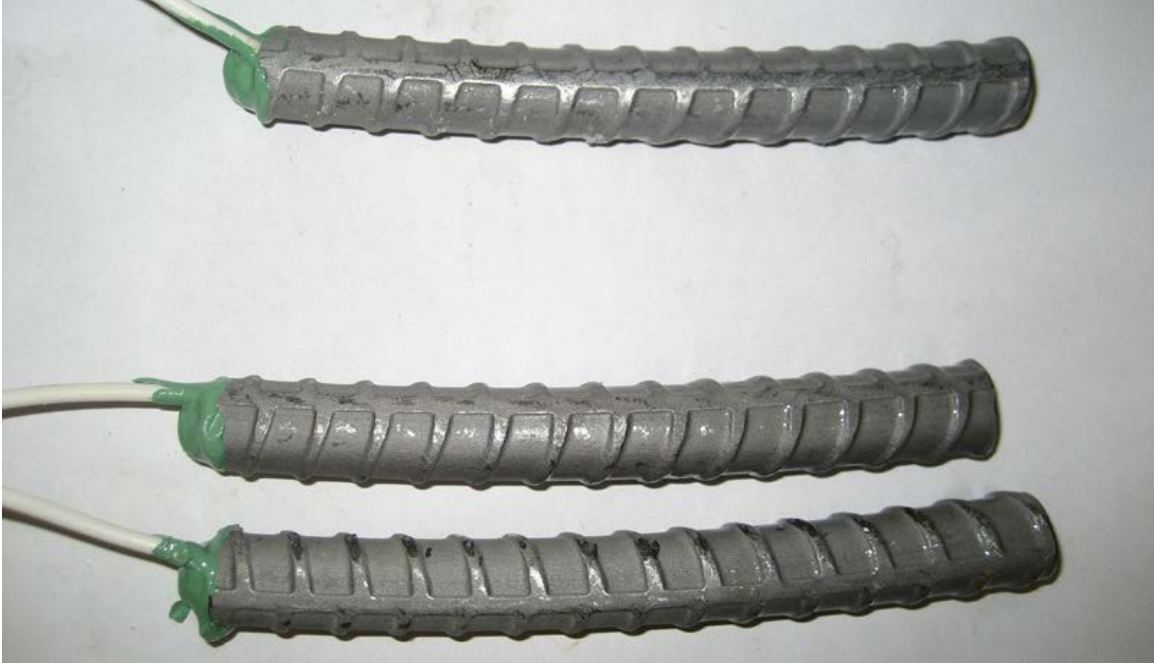
Figure 7: Coiled 2304 stainless steel after testing. Anode (top bar) and cathode (bottom bars).
