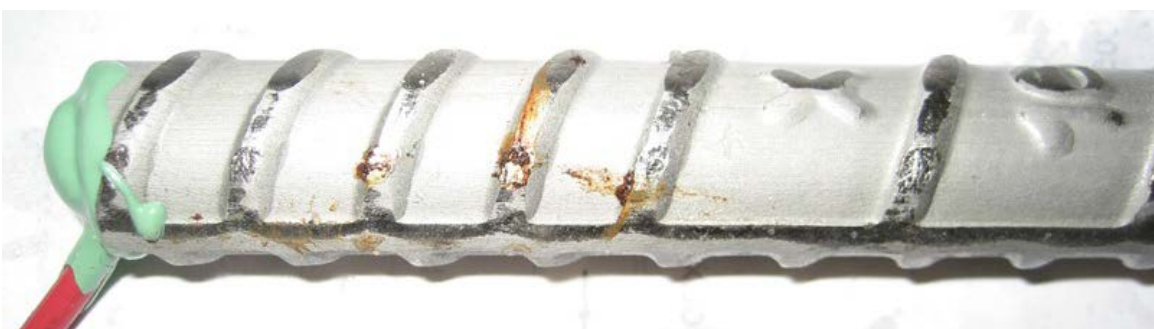
Figure 10b: Close-up of straightened XM-28 stainless steel after testing showing corrosion products on anode bar.
