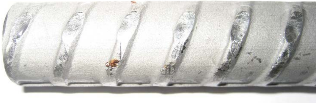
Figure 9b: Close-up of straightened 2304 stainless steel after testing showing corrosion products on anode bar.
